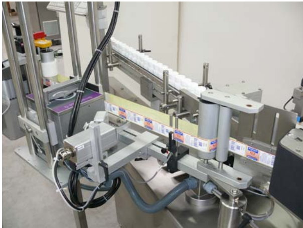
Thermotransfer-Printer and OCV-Camera for verifying the imprint and bar-code
