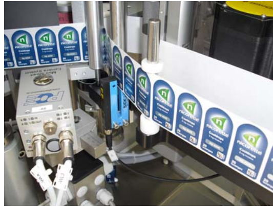
Labelling on 2 sides and vision system
