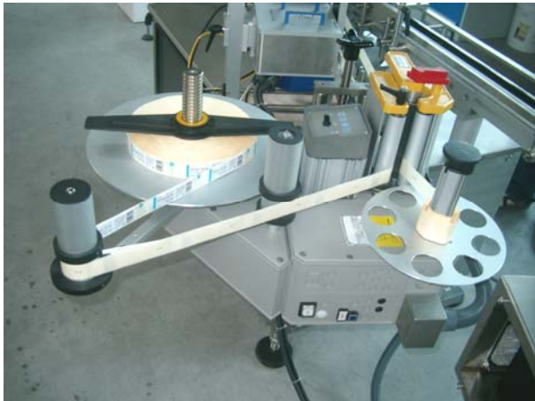
Reel-unwinding and web-collection
